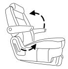
Reclining the seatback can cause an occupant to slide under the seat's safety belt, resulting in severe personal injuries in the event of a collision.
